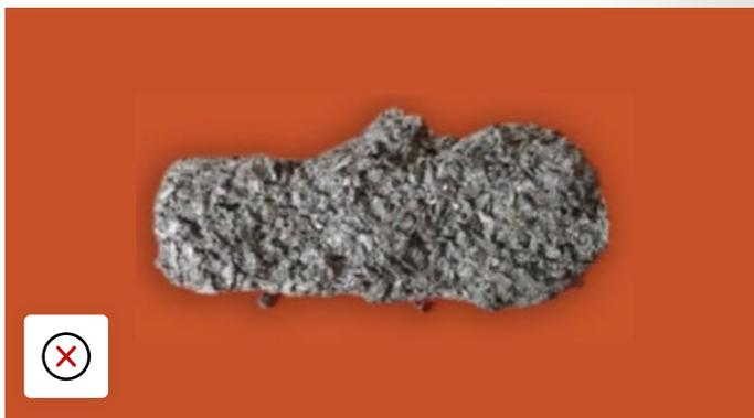
TPMS Sensor contaminated by sealant
