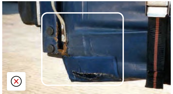
Unrepaired cuts in curtain material at bottom edge.
