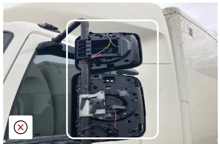
Mirror backing completely missing
