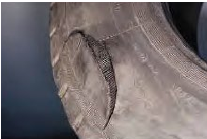
Side wall blow out due to inner line penetration.
