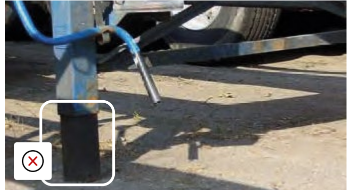
Damage to landing leg cushion foot if not replaced will cause damage to leg inner.
