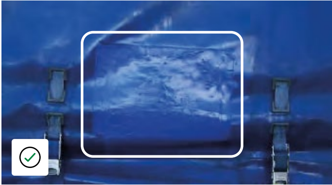
Good exterior panel repair with corners rounded to prevent lifting.
