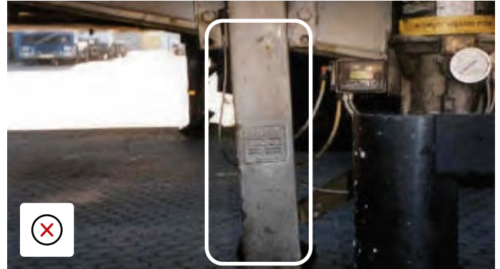
Landing leg bent & needs to be replaced
