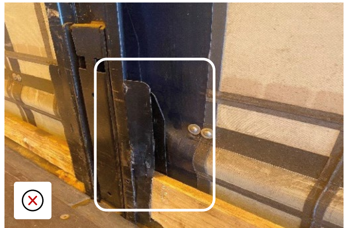
Board holder bracket bent by impact
