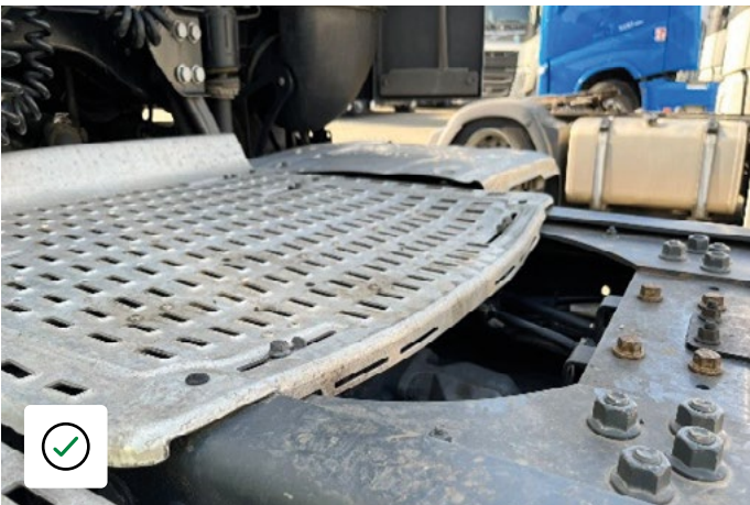
Minor deformation through normal wear & tear
