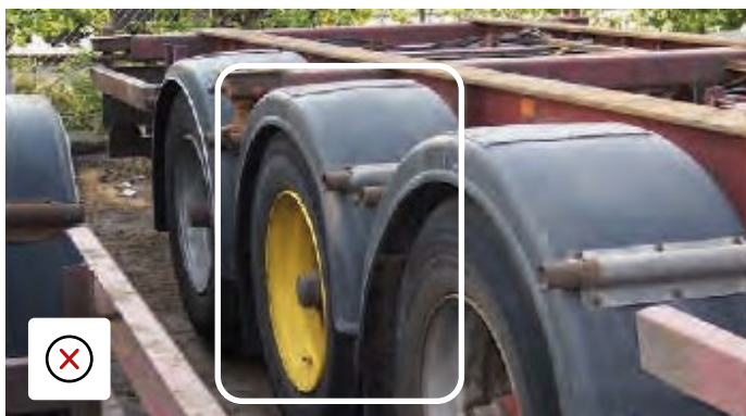
Wrong colour wheel and patched wings, damage possibly due to over loading or being run at wrong ride height.
