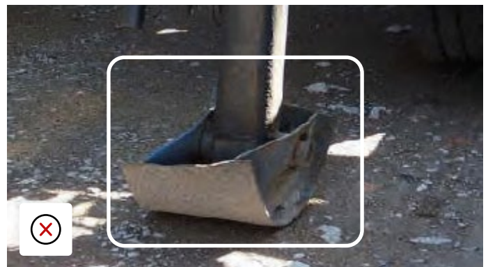
Damage to landing leg swivel foot will be detrimental to the operation and is beyond acceptable limits.
