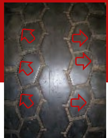
Tread groove cracking due to over inflation
