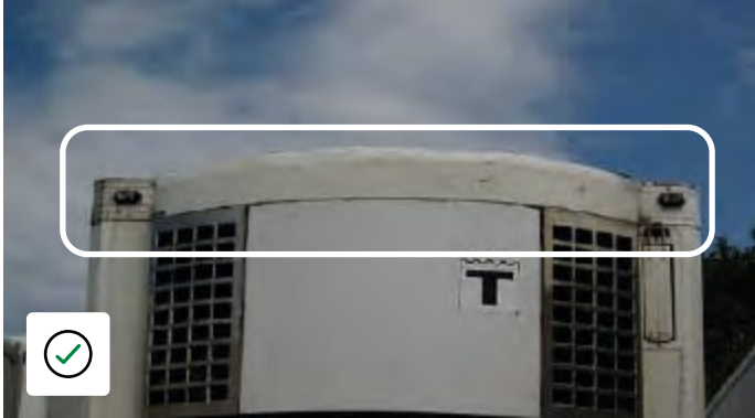
Superficial dents to cowling that do not negatively impact the cosmetic appearance of the unit.
