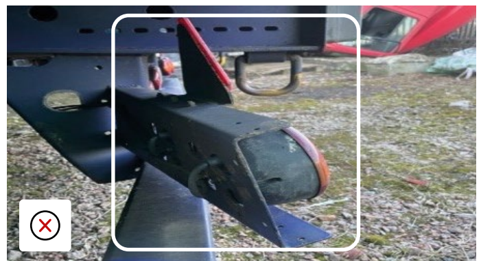
Lamp arm bent & requires repair
