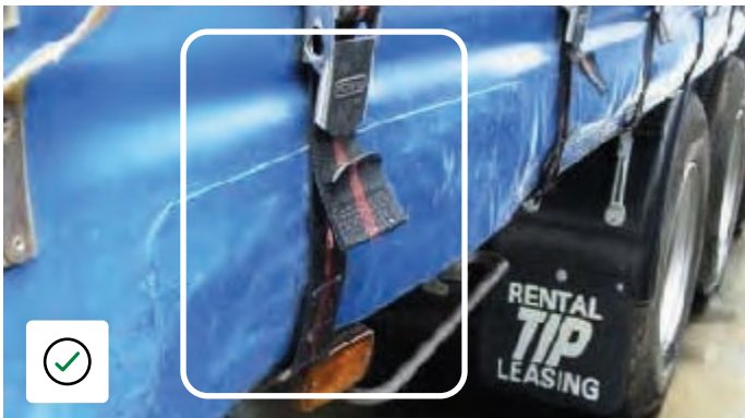
Good exterior lower edge repair with corners rounded to prevent lifting.
