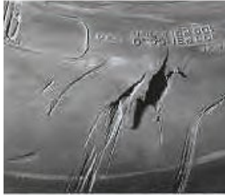
Deep penetration sidewall damage to tyre
