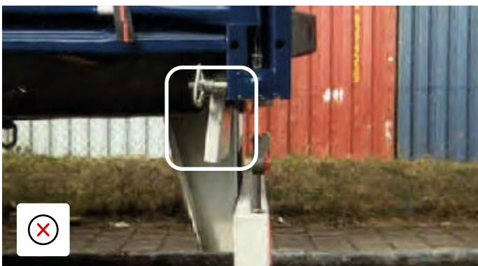
Bent rear lamp girder.
