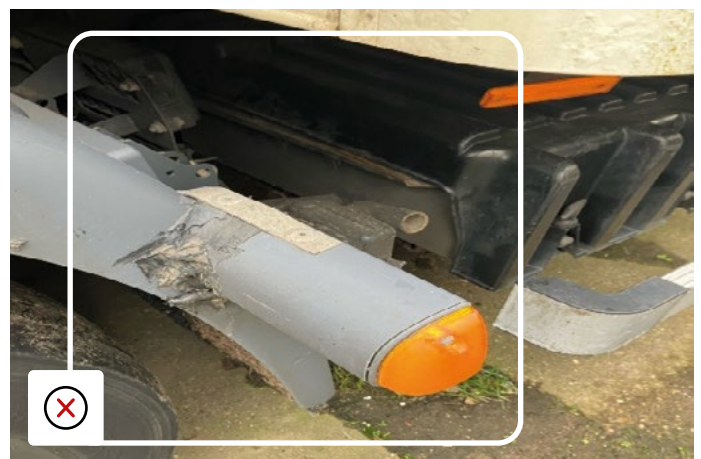
Substandard repair to side repeater mounting
