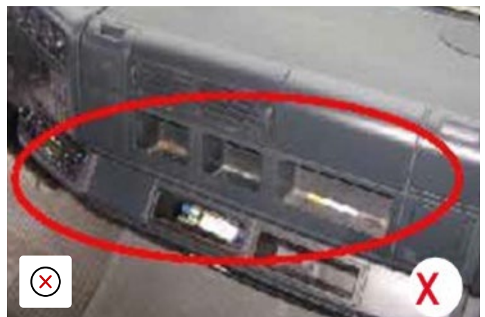
Blanking covers missing
