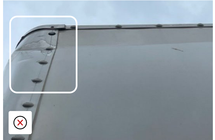
Corner post damaged due to impact with surface paint removed.
