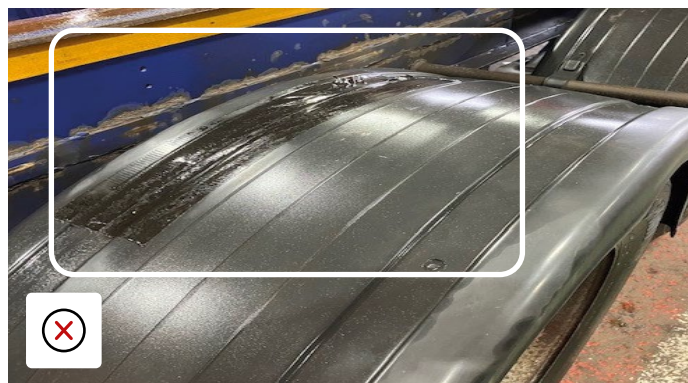
Patched wing requires replacement
