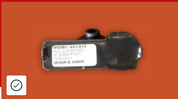
TPMS sensor in an acceptable condition
