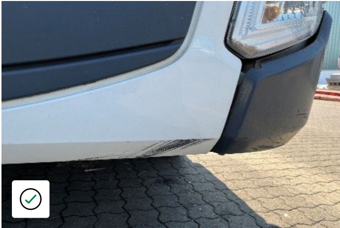
Minor scrape - no damage to the structure
