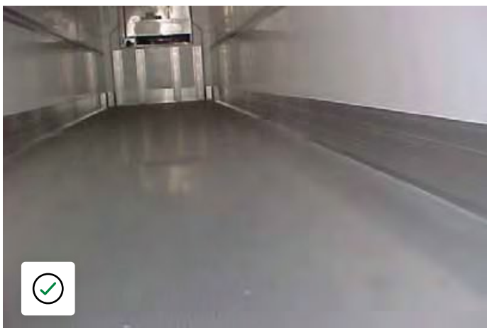
New Floor FW&T does not include excessive distortion splits or holes due to abuse.
