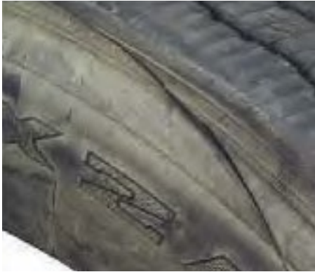
Deep penetration to tyre, shoulder and sidewall damage.
