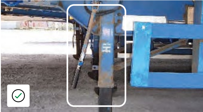
Landing leg straight with handle secure.
