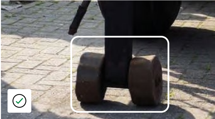
Damage to landing leg wheels and axle but not detrimental to the operation.
