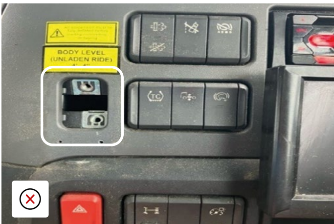
Screw holes in dash & trim missing
