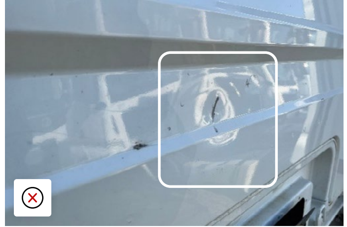
Impact damage to rear of cab causing crack
