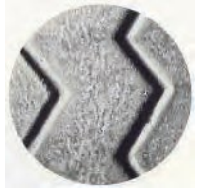
Elephant skin effect or Feathering due to tight manoeuvring creating drag on tyres.
